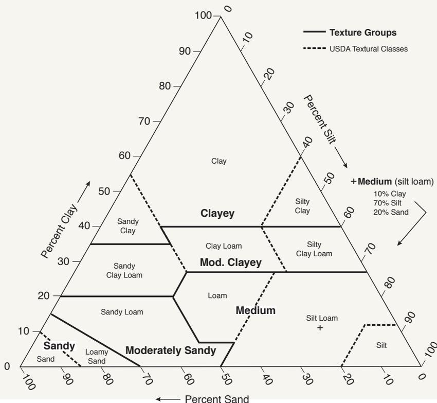
*Figure 4. This soil texture triangle shows texture classes (dashed lines) and soil evaluation texture groups (solid lines). A soil sample located at the + point on the triangle would be composed of 10 percent clay, 70 percent silt, and 20 percent sand. This soil falls in the medium texture group and the silt loam texture class.*
