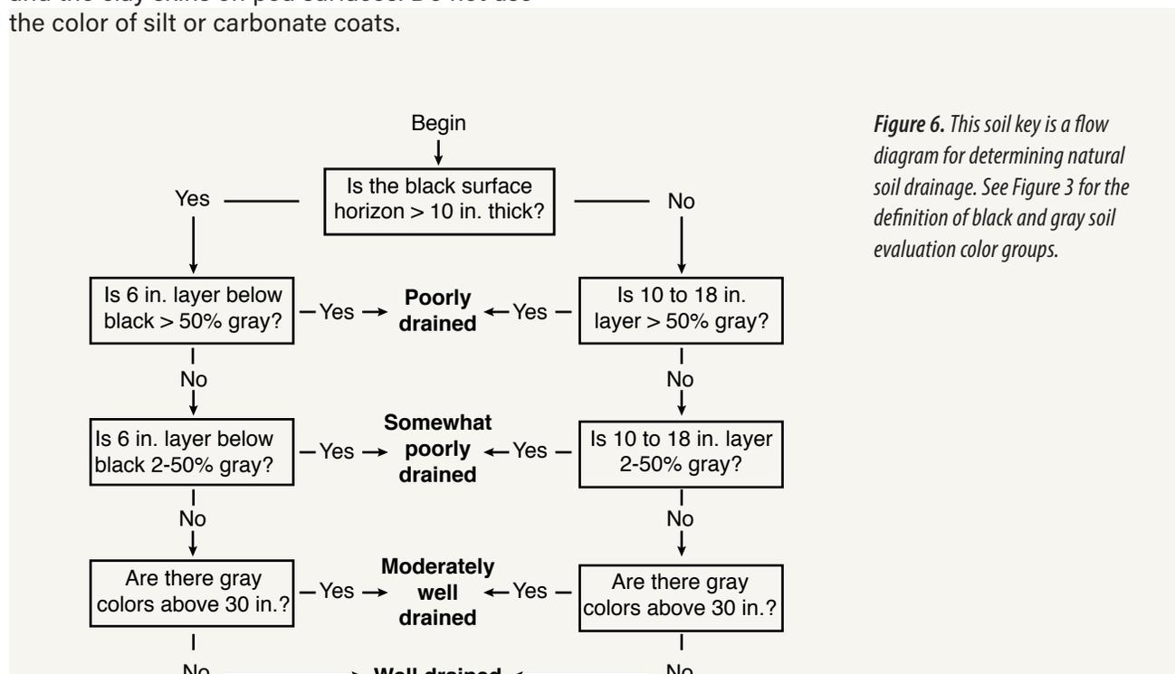
Figure 6. This soil key is a flow diagram for determining natural soil drainage. See Figure 3 for the definition of black and gray soil evaluation color groups.
